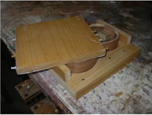
With the body completely flat I went to work with my sanding sheet. It was reasonably easy to tell when to stop – I had left the linings and sides a little proud of the neck and heel blocks, and when I could see that I was sanding the tops of the blocks I knew I was close to finished.
