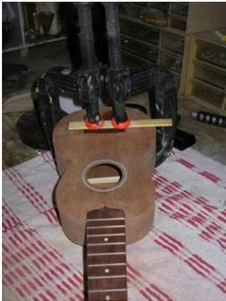
I lightly sanded the bottom of the bridge, as some wood had been pushed out of the screw holes when they were drilled, causing a slight bump that would have prevented full bridge contact with the soundboard.
