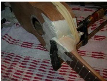
Once the neck was in the right position, I drew a pencil line either side and around the end of the fretboard and masked the area. After that, I applied glue to the neck and clamped it on with a screw clamp and rubber bands. This was
