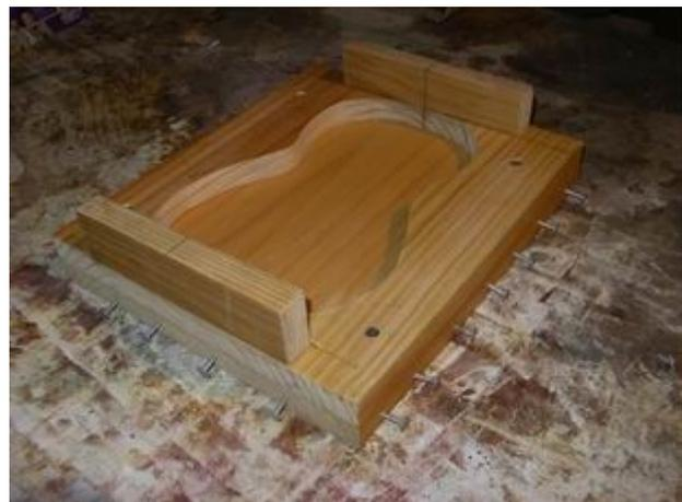
In the second picture, nails have been placed around the edge of the base. These are used to anchor the rubber bands used for clamping (the bands are supplied with the kit). Note the centreline marks on the jig.
