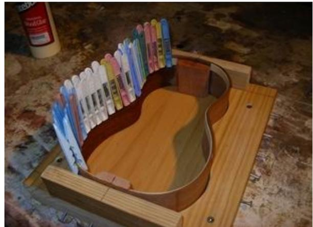
After the back linings are glued in, flip the uke over in the mould and glue in the linings for the soundboard (top).
