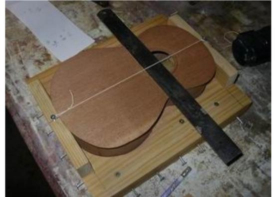
Making sure that the top centre line aligned with the centrelines at both ends of the mould, I held the top down with one hand and ran a pencil around the underside of the top. I then took out the
