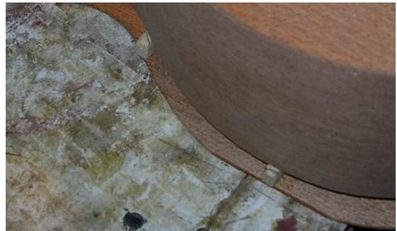
away brace wood and glue residue from the ply. I then tried to fit the back (note that I had also marked on the uke sides where the braces should be located). At first it wouldn't go, but with a very fine trim to the ends of both braces it went home with a satisfying click. After that, I carved the braces down at the ends with a sharp knife and sanded them clean.
