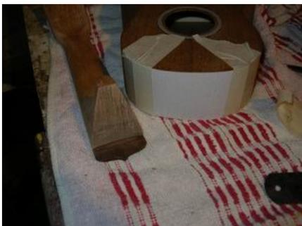
An important prep is to remove any glue residue that may have oozed out of the joint between the fretboard and neck. I used a sharp blade. Then I taped sandpaper to the body and scribbled pencil on the neck gluing face of the neck, and worked the neck back and forth until most of the pencil marks had gone, indicating a flush fit.
