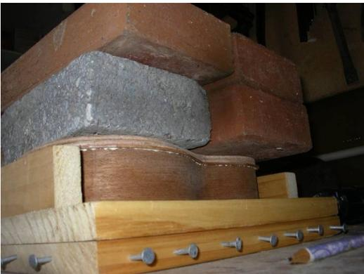
top, turned it upside down on a flat wooden surface and trimmed it close to the line with a sharp knife, using a straight edge to make sure that the knife did not slip
