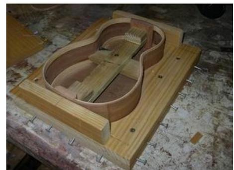
I also made up a new insert for the mould, just 4 mm thick. This raises the body enough to sand, but keeps it well within the mould. I also screwed the whole mould and base to my workbench, to stop the uke slipping around while I sanded it. Do not try this if you are building the uke on the kitchen table!!
