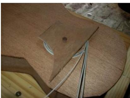
The swelling was addressed by a light sand either side to reduce the width of the glued strips. To decrease the number of fingers needed to hold the rosette, I made a spider affair (from a plywood scrap – just happened to be a good design!) and fastened it to the block under the sound hole with a screw. Tightening the screw pulls down the ply and keeps the rosette where it ought to be. In the earlier picture, the piece of ply is sitting on the uke top but has not yet been screwed into the
